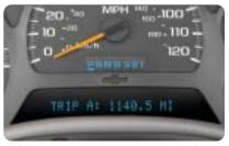
The DIC display is located above the steering wheel on the instrument cluster, and can be programmed in three languages. The controls are located on the steering wheel:
